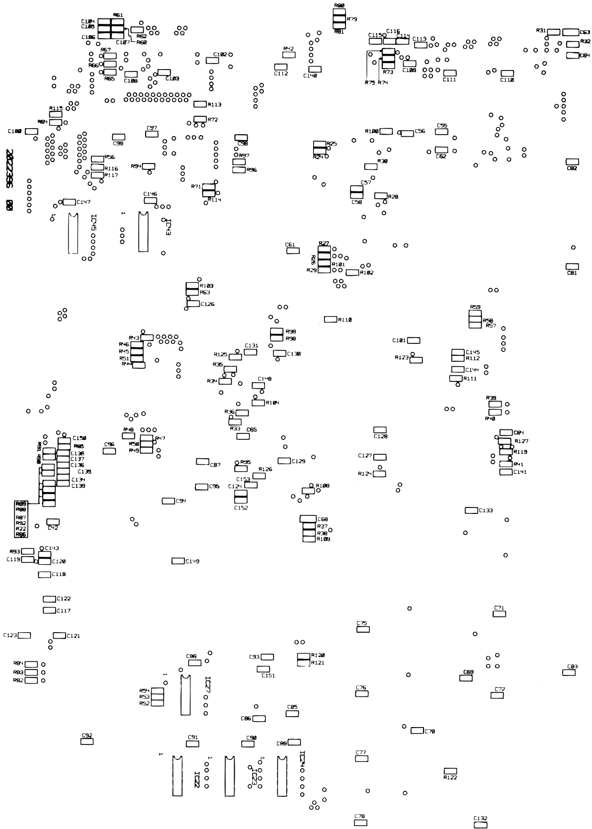
Figure A-14. C207 MAIN Board Component Layout (Rear)
